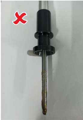
Fibres and dirt sticking on the spindle blade
