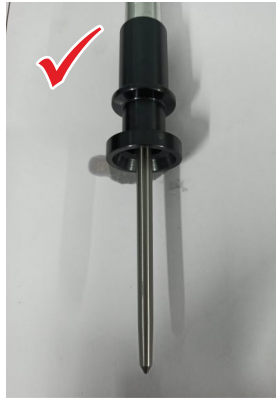
Clean spindle blade
