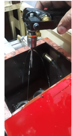
Neck bearing oiling method
