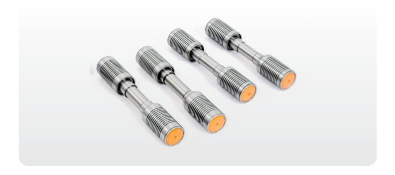
op rollers consist of a pair of anti-friction, double row ball bearings with a common axle. Each top roller is manufactured such that the clearance between the hardened arbour and shell is perfectly matched with appropriately sized double row steel balls. The top rollers made for ring frames and speed frames are injected with just the right amount of a special grease – TRG 5. The ends are fitted with a uniquely designed seal to prevent leaks while in operation.
