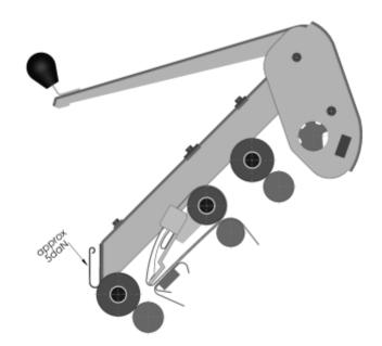
Weighting arms PK 1601-01 are equipped with a partial load relief feature (please refer figure above). Opening the hand lever to its first rest position activates partial load relief. When the machines are going to remain idle for a long time, one can use this feature to release the front top rollers with load reduction to 5 daN.
