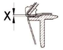
The vertical distance between the nose bar and the cradle at the nip point (distance 'X' in the figure above) determines the intensity with which the fibres being spun are controlled and guided between the top and bottom aprons in roving frames as well as in ring frames. To achieve optimum drafting conditions, the opening 'X' can be adjusted using distance clips to achieve best quality of yarn (in ring frames) and roving (in roving frames).
